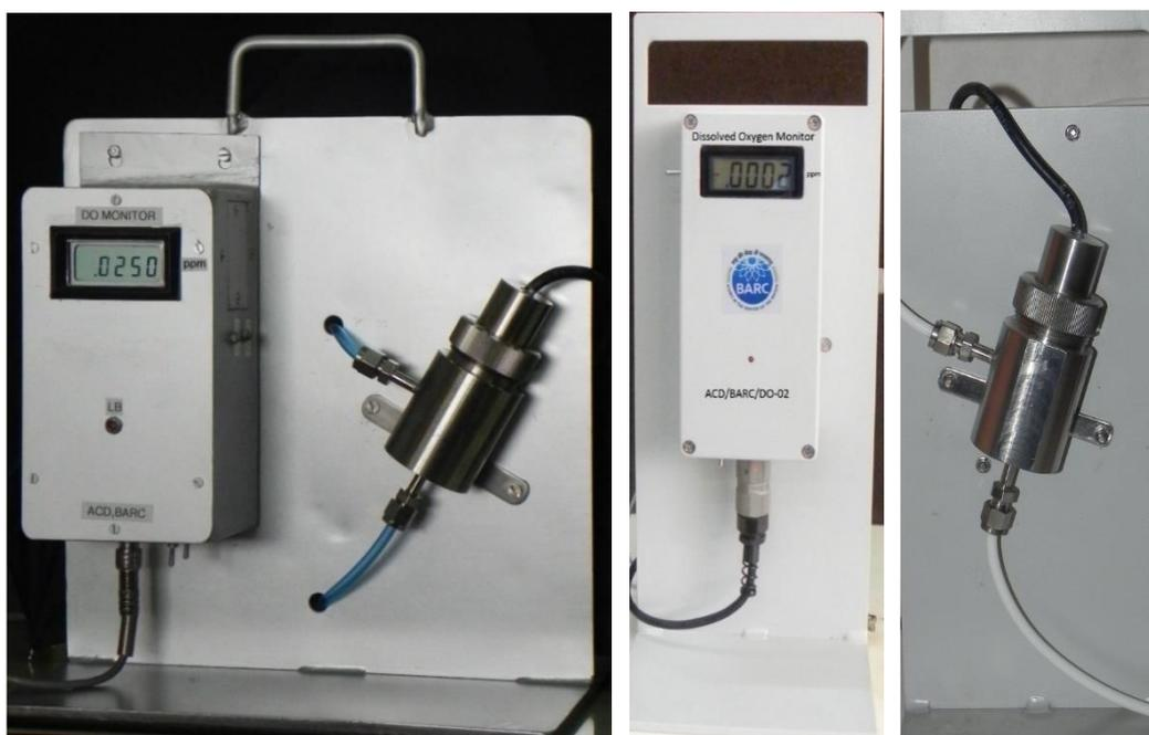
Figure 3. Picture of the dissolved oxygen monitor which has been developed and technology has been transferred to several companies, Technology code: CH32ACD, Website, <http://barc.gov.in/technologies/dom1/index.html>.
